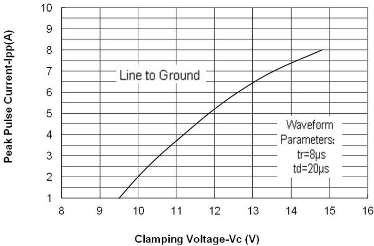
**Fig. 3 Clamping Voltage vs. Peak Pulse Current**
